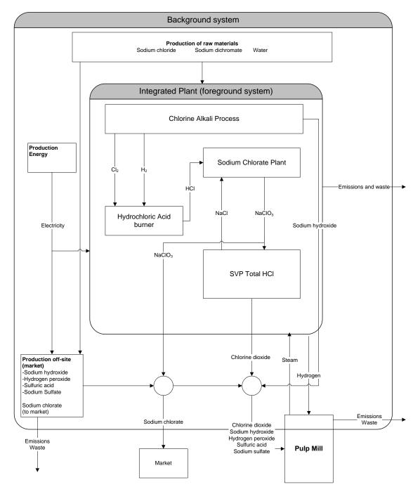
Figure 4 The integrated plant foreground and background systems
